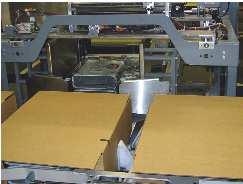
Two clamshells containing Xbox 360 game components are stacked one on top of the other and the two units are pushed into an end-loading shipping case.
