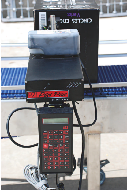
A case printer imprints the sealed wine case with bar-code information.
