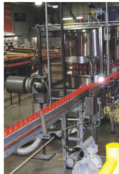
A long, U-shaped section of conveyor after the bottle unscrambler/orienter provides accumulation ahead of filling.
