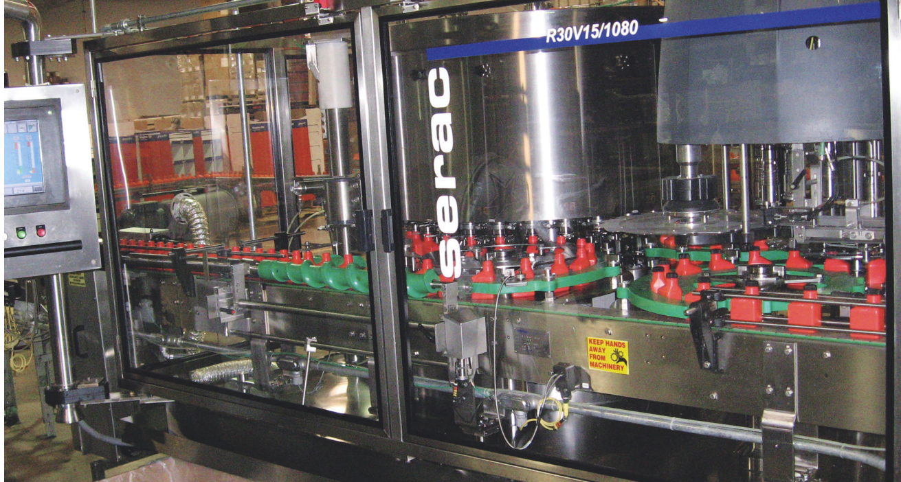
Monobloc netweight filler/capper with 30 fill valves and 15 capping heads runs bottles ranging in size from 2.6 to 20 oz.
